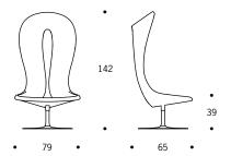
design: busk+hertzog • fabrics: optional • materials: high-quality moulded foam - aluminium swivel base with powder lacquer all dimensions in cm - we reserve the right to make alterations to the model
